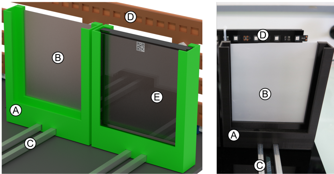
Figure 5: Plate support. Annotated 3D rendering (left) and picture (right) of the plate support. The U-shaped plate support (A) carries a diffusion filter at the back (B) allowing an homogeneous near-infrared illumination. Each support moves horizontally on the double axis (C). A classical 12.5 cm x 12.5 cm square plate fit into the plate support (E).
